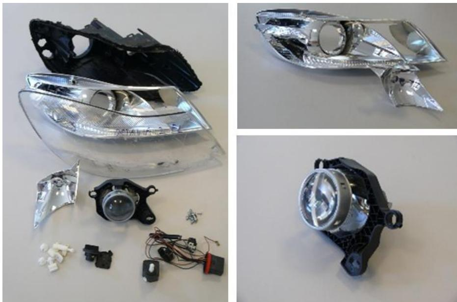
**Figure 3: Decomposition of the front light of the Skoda Octavia of the 2nd generation**
