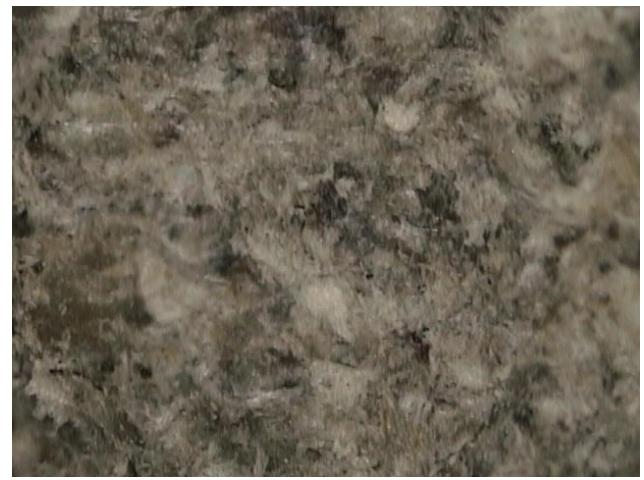
d) zoom view (40x) to the pellet surface along the axis-sample 2
