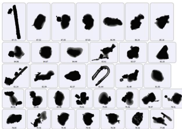
**Figure 3: Shapes of particles the graphite dusty waste**
