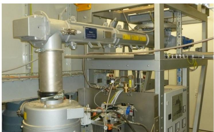
Figure 3: Paddle homogenizer with water jet
