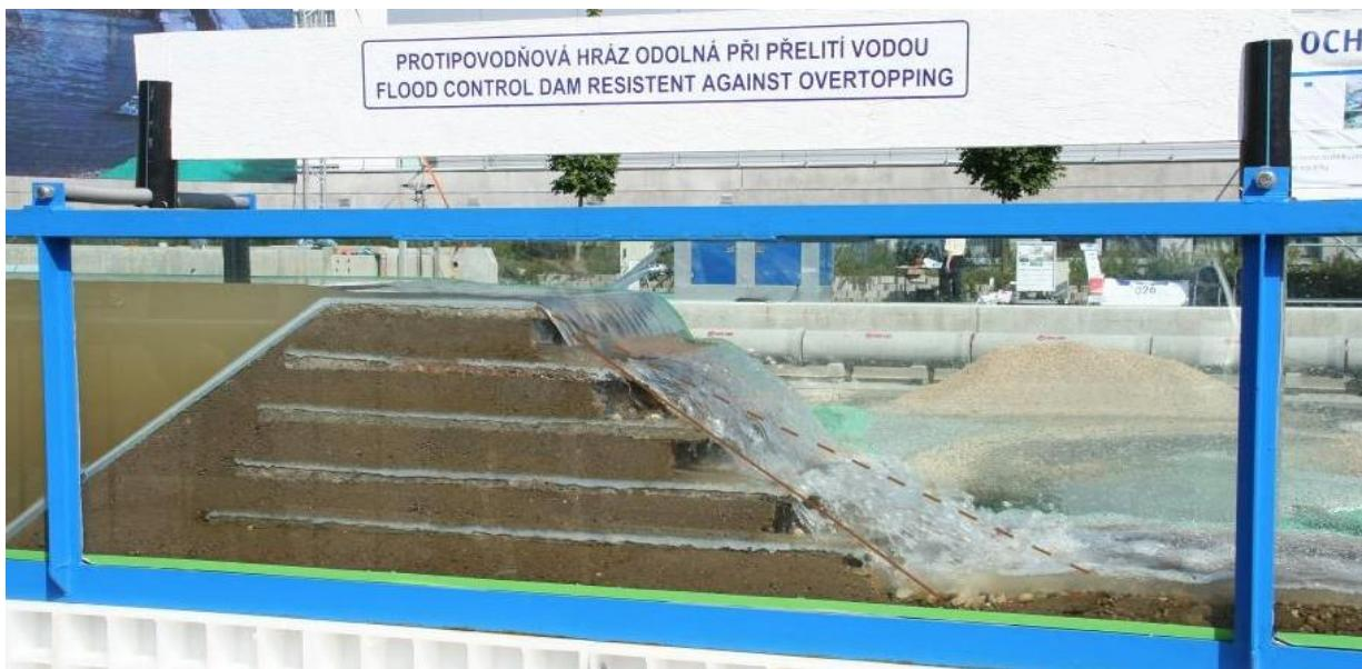
Figure 3: Flood control dam resistant against overtopping – model
