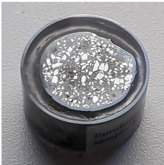
Figure 8: Cut through the sintered tungsten sample.
