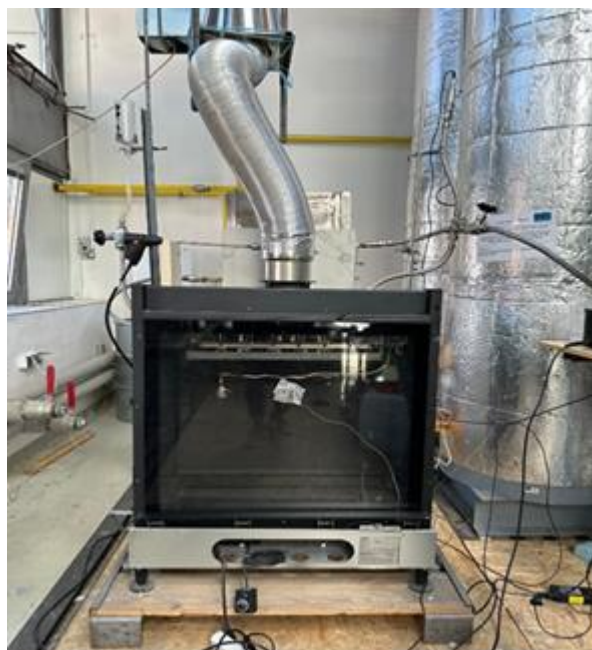
Figure 4: Real setup of the fireplace with heat pipe
