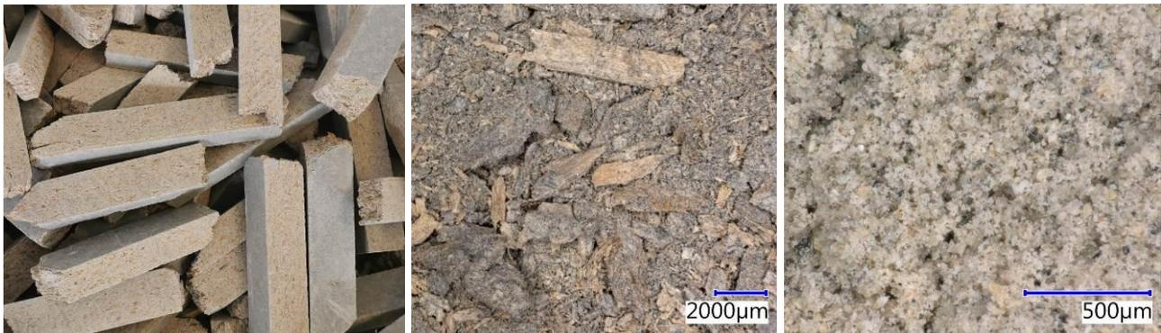
**Figure 1, 2 and 3: Cuttings from cement-bonded particleboards – raw (Fig. 1 - left), after crushing in a jaw crusher (Fig. 2 – middle; image from optical microscope) and separated grains of 0-63 µm (Fig. 3 – right; image from optical microscope)**
