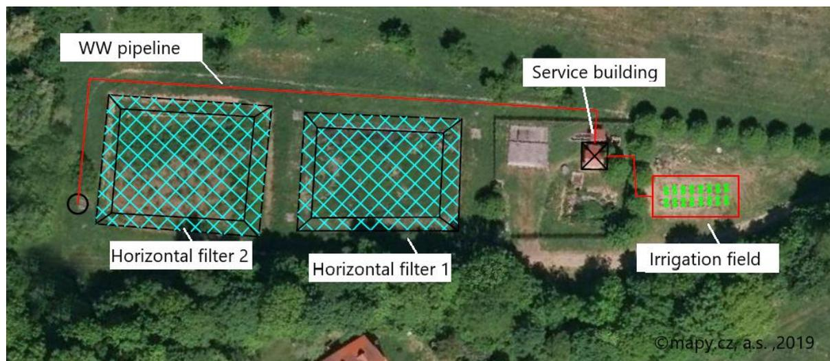
**Figure 1: Schematic image of the experimental location**
