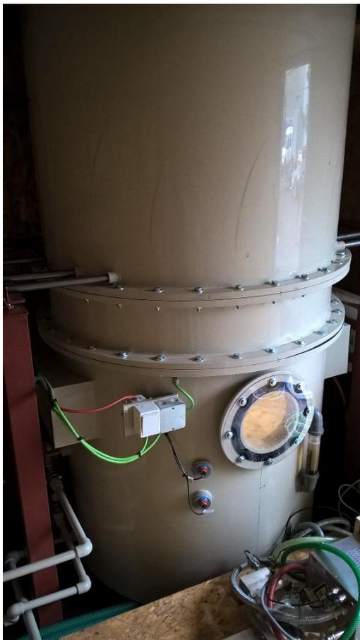
Figure 8B: Body of biotrickling filter
