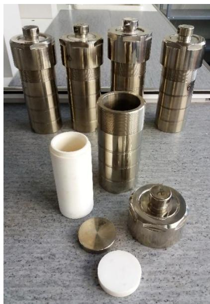
Figure 3: Autoclaving capsules
