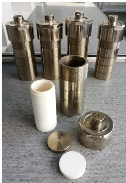
**Figure 3: Autoclaving capsules**
