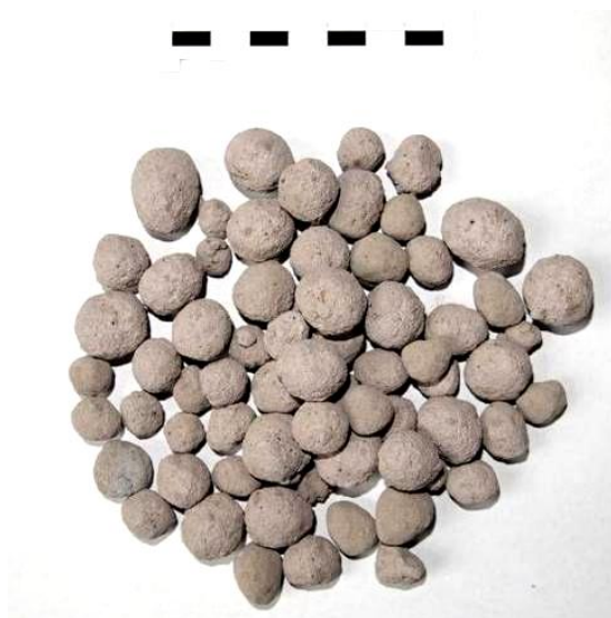
Figure 2: Grain from the granulation plate (already free of moisture)
