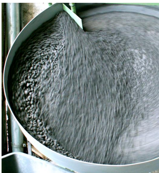
Figure 1: Granulation plate in operation at the optimum setting
