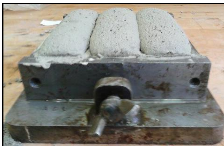
Figure 1: The typical appearance of the fresh mixture in a mold
