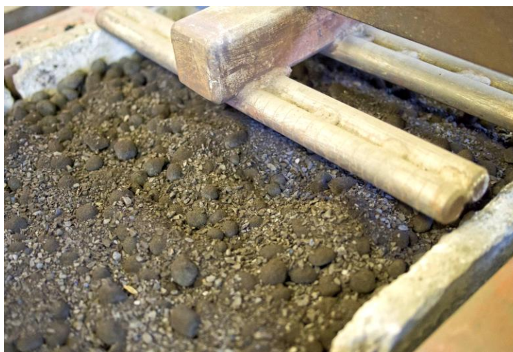
Figure 4: Fresh batch with ignition layer
