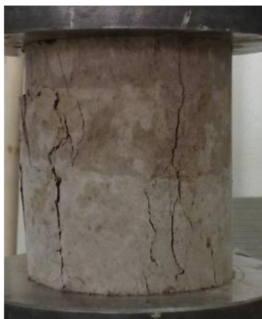
Figure 8: Crushed solidification product NS2-E at UCS test (subjected frost resistance test)
