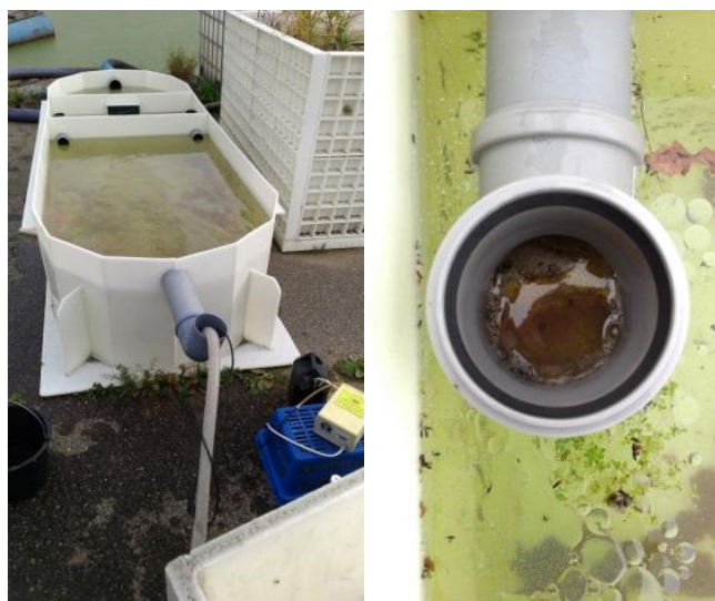
Figure 2a and 2b: Semi-operated model of DUN stormwater tank (left). Accumulation of oil substances at on the water surface during validation testing (right).
