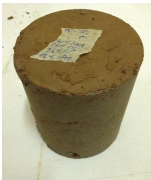
Figure 7: Solidification product NS1-D after frost resistance test
