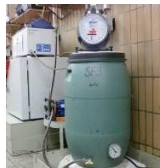
**Figure 3: Fermentor for the model test 3**
