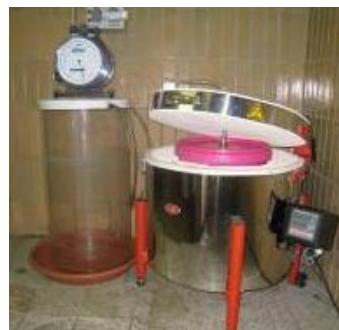
**Figure 1: Fermentor for the model test 1**
