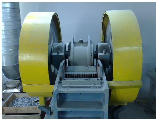
Figure 3. Semi-industrial L44.41 jaw crusher with complex jaw's movement produced by Makrum, Poland
