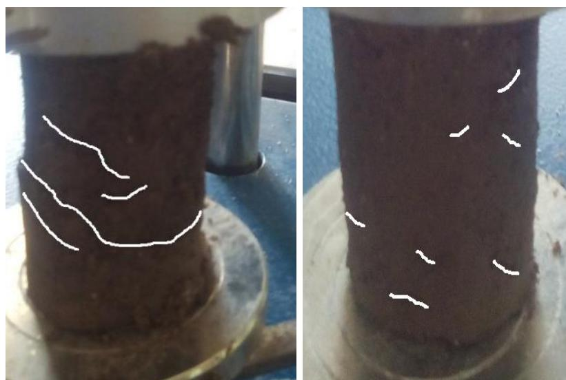
**Fig.7: Stabilized sample after compressive strength test. (Left): the sample stabilized with 14% of the mineral wastewater content and (Right): the sample stabilized with 35% of the mineral wastewater content**
