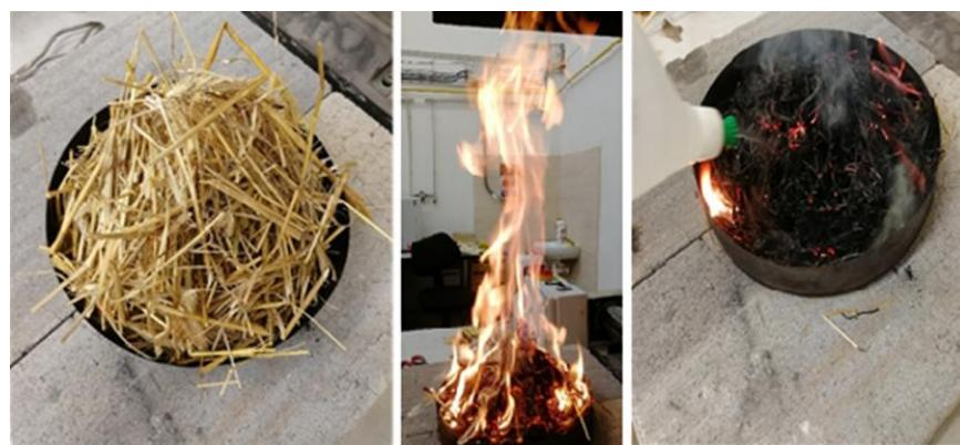
**Figure 2: The process of sample preparing: sample of straw, simulated full developed fire, fire extinction (from the left to the right).**
