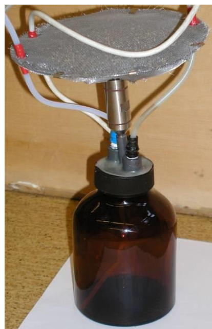
Figure 1: Scheme of the seeping water sampler and photograph of the sampling bottle, valve and “area lysimeter” 16,9
