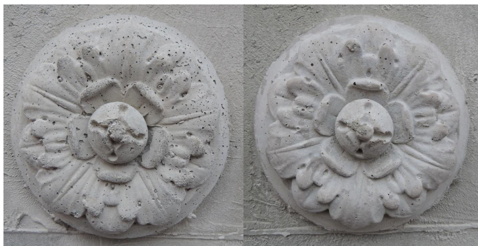
Figure 2: Detail views of the Desil AL (left) and DVS2 rosettes (right) after 360 days on the facade
