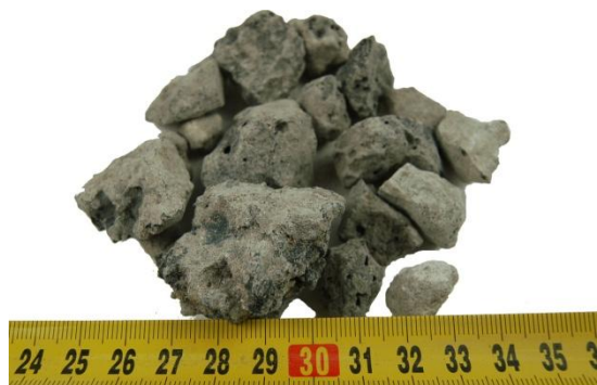
Figure 16: Blended Ladle slag, sample 6
