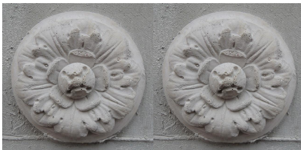
Figure 3: Detail views of the NaVS1.5 (left) and MKS rosettes (right) after 360 days on the facade
