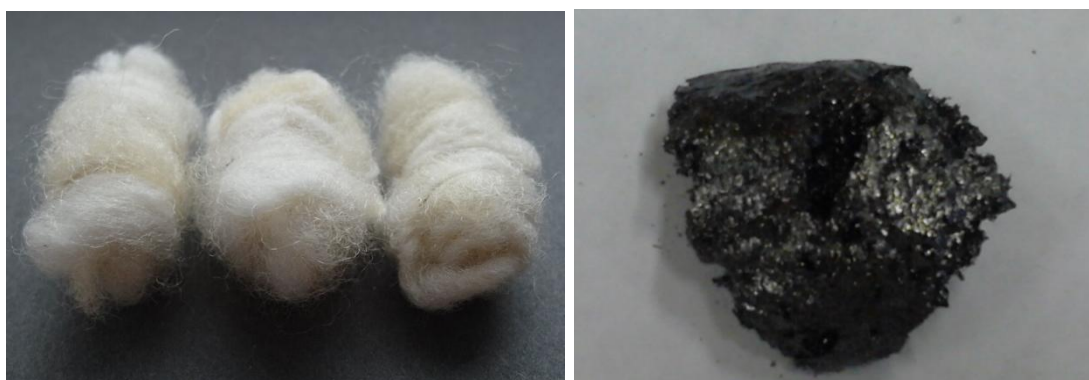
Figure 1: Wool prepared for pyrolysis (left), sheep wool pyrolyzate (right).
