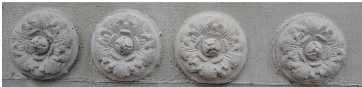
Figure 1: Comparison of rosette appearances after 360 days on the facade
