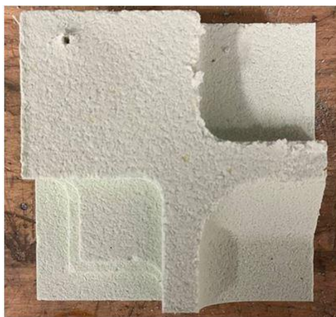
Figure 10: Machined SB-0140 block pressed at 4.9 MPa.
