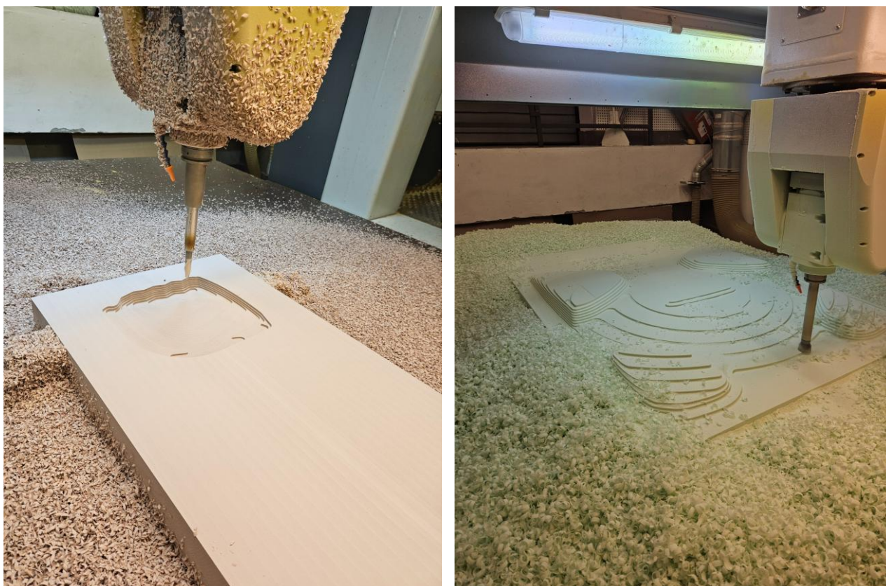
Figure 1: Chips from CNC machining of PU tooling boards.
