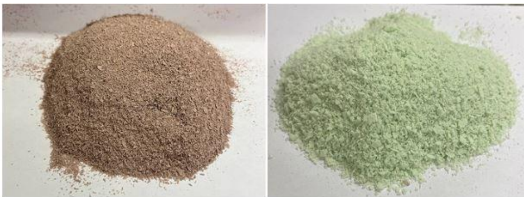
Figure 2: Crushed PU feedstock: SB-0600 (left) and SB-0140 (right).
