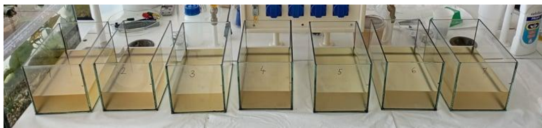
Figure 2: Leachates prepared by 24-hour leaching (Photo: H. Hybská)
