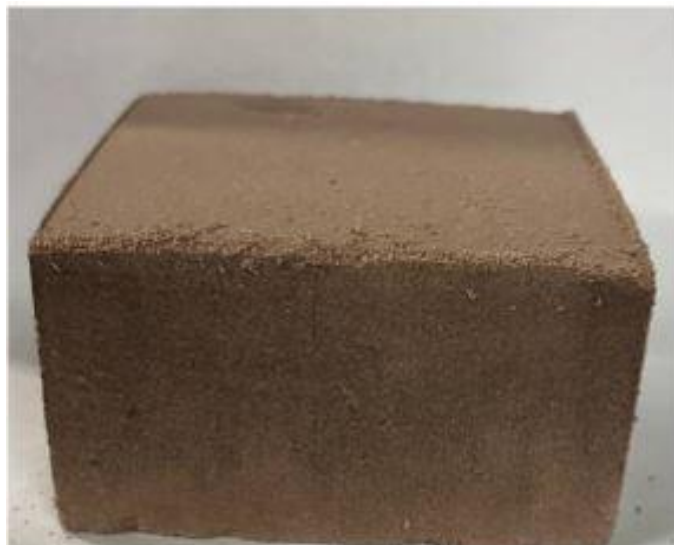
Figure 6: Cold-pressed block from crushed SB-0600 chips with binder.
