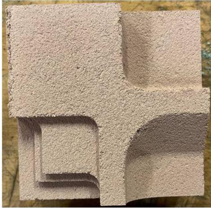
Figure 11: Machined SB-0600 block from crushed feedstock pressed at 14.7 MPa.
