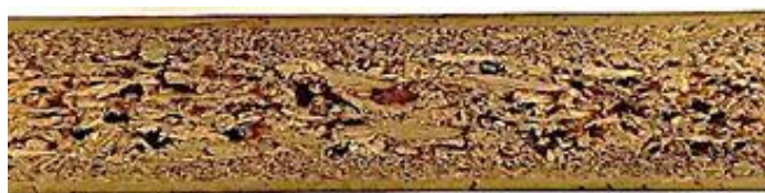
Figure 1: Three-layer particleboard with incorporated polymer (Photo: V. Mancel)
