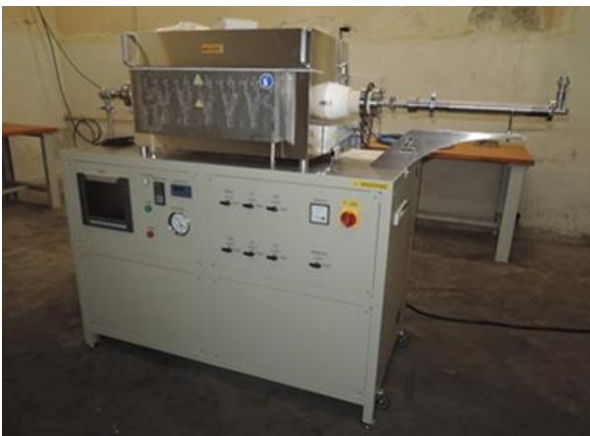
Figure 8: Laboratory refining equipment for the thermal treatment of metallurgical waste
