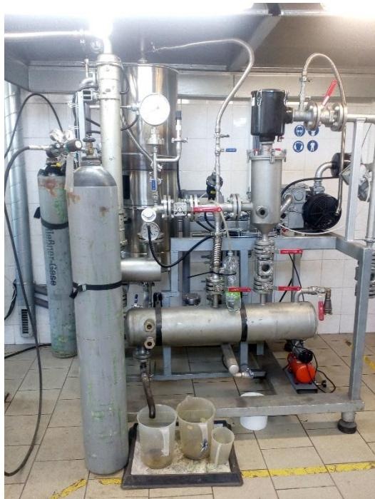
**Figure 6: Part of Thermal Desorption Technology - Condensing Unit and Collection of Compounds in Liquid Phase.** Source: Authors
