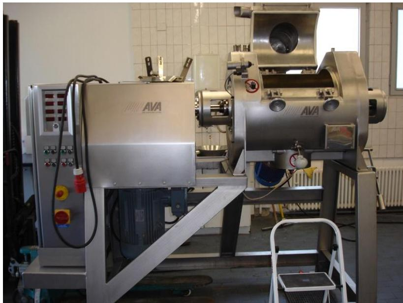
**Figure 3: AVA Thermal Desorption Laboratory Unit.** Source: Authors
