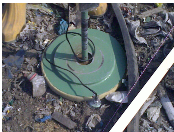
Figure 1: The pictures show the experimental sampling adapter (left) and the landfill surface simulator, including the gas piping system (right).
