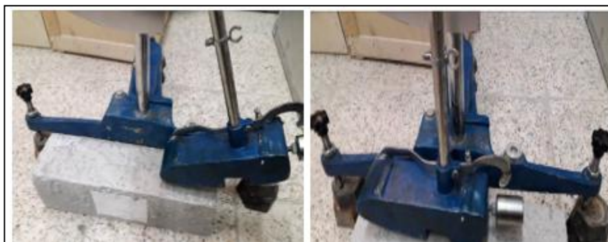
Figure 2: Sample of concrete surface under British pendulum test
