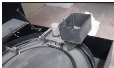
Figure 3: A view of concrete sample surface in Dorry test
