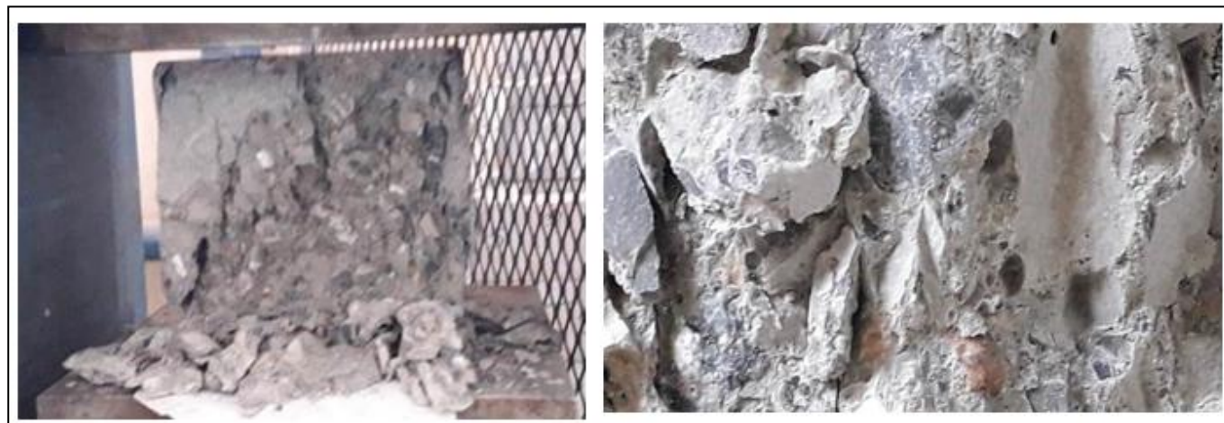
Figure 5: Images showing the cracks propagation in compressive samples
