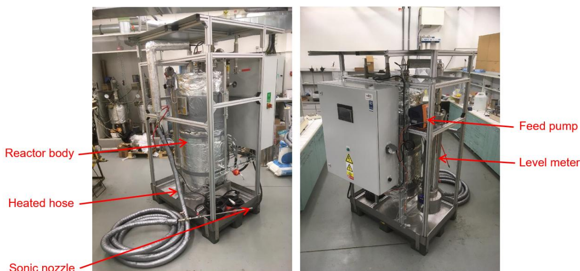
Figure 2: The semi-operational urea hydrolyser
