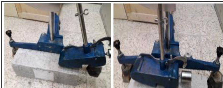
Figure 2: Sample of concrete surface under British pendulum test
