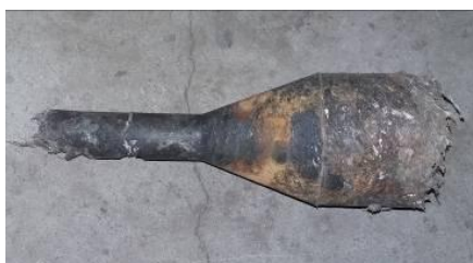
Figure 4: Stopper clog removed from the machine when the frame was cleaned
