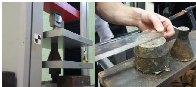
Figure 5: Uniaxial compressive strength test of the clog
