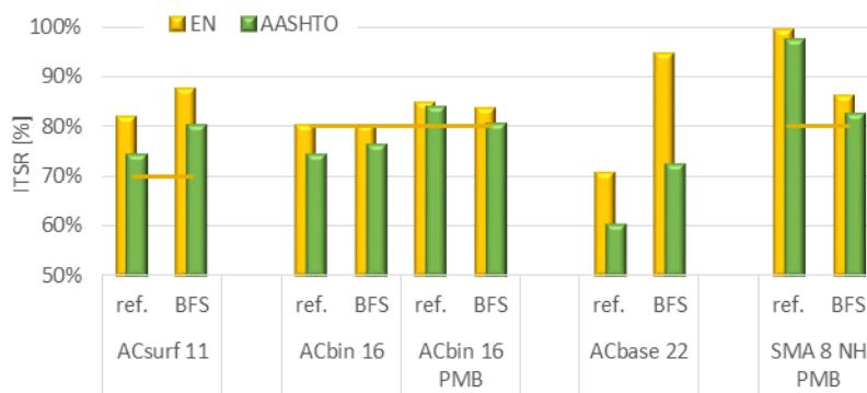
**Figure 4: Indirect tensile strength ratio - ITSR**
