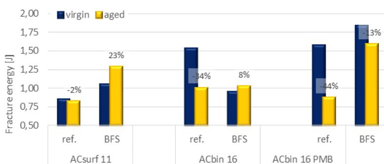
Figure 12: Fracture energy of virgin and aged specimens
